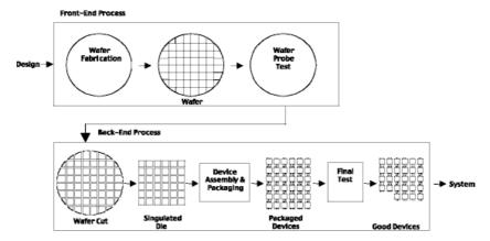
In view of the increasing complexity of semiconductor fabrication, manufacturers have introduced technologies to increase yields and minimize costs. In the front-end process, for example, manufacturers are using metrology and inspection tools to identify, diagnose and minimize fabrication defects. Manufacturers also perform parametric test to verify process uniformity and capability. These tools confirm compliance with some
