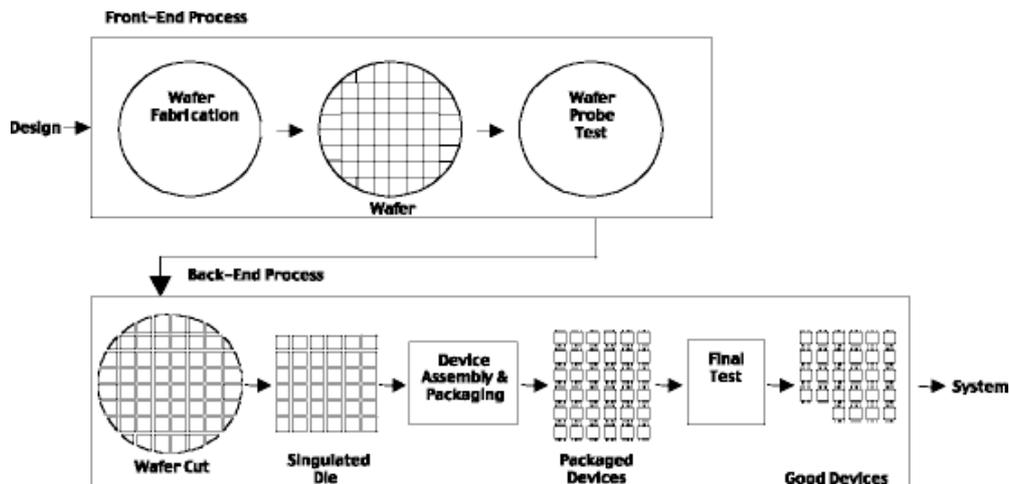
In view of the increasing complexity of semiconductor fabrication, manufacturers have introduced technologies to increase yields and minimize costs. In the front-end process, for example, manufacturers are using metrology and inspection tools to identify, diagnose and minimize fabrication defects. Manufacturers also perform parametric test to verify process uniformity and capability. These tools confirm compliance with some
